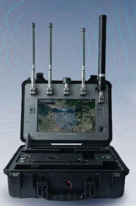
Bluvec's signature product powered by DSI GEN-2. Designed as a portable solution for early-warning, drone detection, identification and location of the drone and the pilot. Blucase's monitoring data stream enables users to data, including the drone model, serial number, speed, geolocation, latitude and longitude, movements of the drone, as well as the pilot's geolocation.
